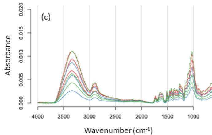
**Figure 3.** Representative FT-IR spectra in the range 4000–650  $\text{cm}^{-1}$  for Alaska yellow cedar samples according to durability classifications established by exposure to (a) *G. trabeum*, (b) *R. placenta*, and (c) *R. flavipes*. Green = highly resistant, blue = resistant, red = non-resistant.
