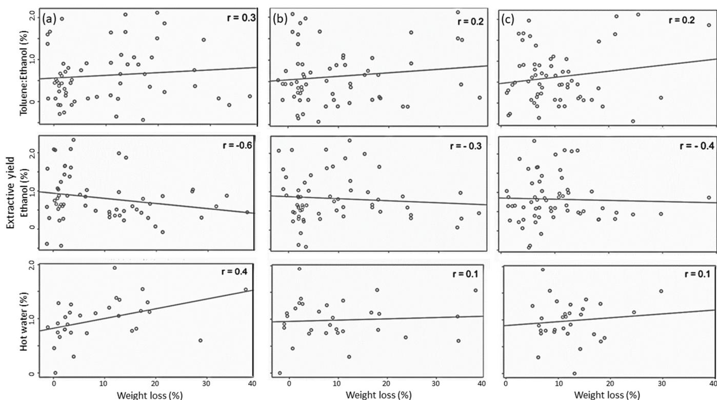
**Figure 2.** Relationship between weight losses (%) caused by exposure to (a). *G. trabeum* (Gt), (b). *R. placenta* (Pp), and (c). *R. flavipes* (Rf) and extractive yield using three different solvents: hot water (bottom), ethanol (middle), and toluene-ethanol (top).
