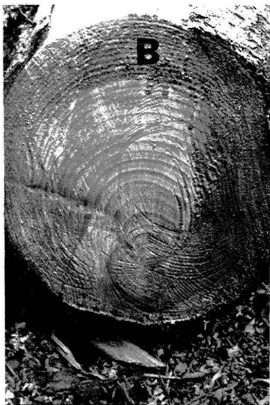
Figure 22.—Compression wood is common in leaning and crooked white pine trees. A, severe lean in a white pine tree. B, a cross-section of the leaning portion of the tree, showing eccentric growth rings with compression wood.
