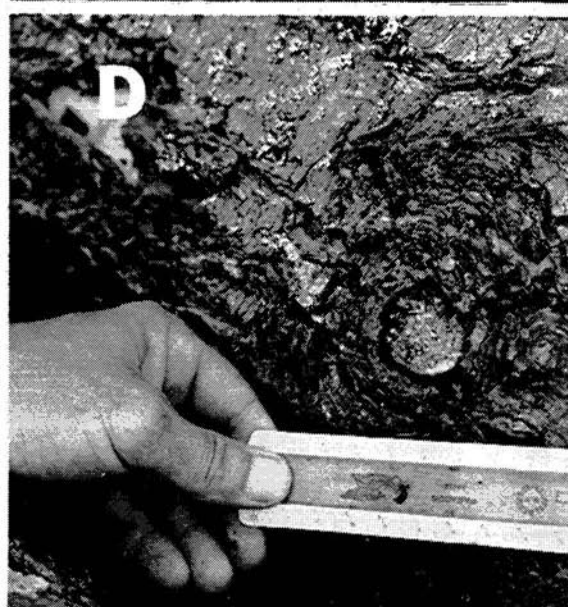
Figure 3.—Dead log knots on white pine logs. A, a sound dead log knot showing no signs of deterioration. B, a dead log knot showing moderate signs of deterioration. C, the same knot chopped out to a depth of 3 inches and still showing encased condition. D, an unsound dead knot showing advanced deterioration.
