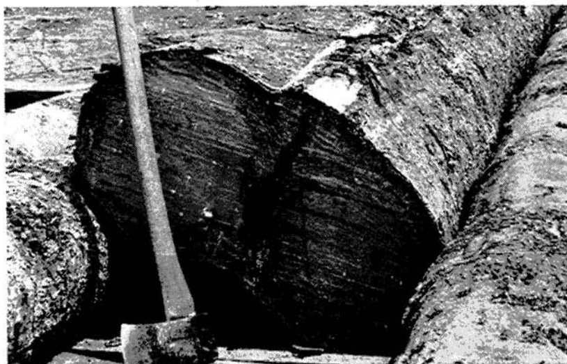
Figure 20.—Bark seam in log, caused by forked tree.
