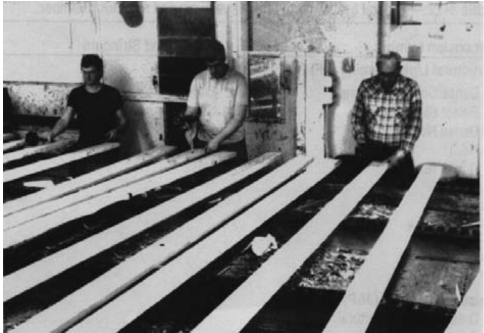
Figure 3-26.- Sawn lumber being visually graded and marked at a sawmill (photo courtesy of Funk Lumber Co.).
