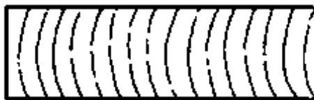
Edge-grain plank; rings form an angle of 45° to 90° with the wide surface.
